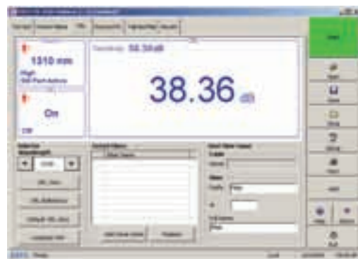
The FTB-3930 comes standard with a high-accuracy ORL meter.
